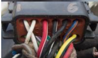
2004-06 Sportster Harness 12-Pin Deutsch Connector WHITE Jumper Wire (Pin2) used for TC80A Programming
