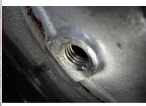
Before drilling, the hole was packed with grease and a small piece of stainless was put on the other side to keep from drilling anything and (hopefully) stopping some of the chips from falling further into the engine.
