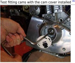
On a 2003 or older motor, you can verify cam fit by installing all 4 cams without the pinion gear in place and then turning them from the rotor cup screw. They should turn freely, without binding.
