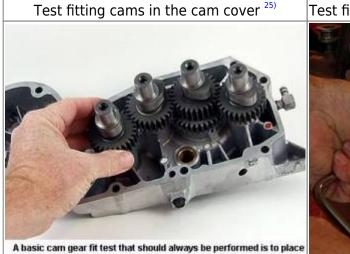
A basic carn gear fit test that should always be performed is to place all 4 carns into the cover and make sure they turn without binding. This test should also be repeated in the crankcase. Note the cut down carn cover above.
