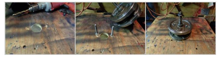
Use a 1-5/16" socket wrench to remove the crank pin nut on the sprocket side. With the crank nut off, lower the all-thread below the top wheel and retighten the nuts. You'll be knocking the top wheel sideways next to loosen it from the crank pin.
