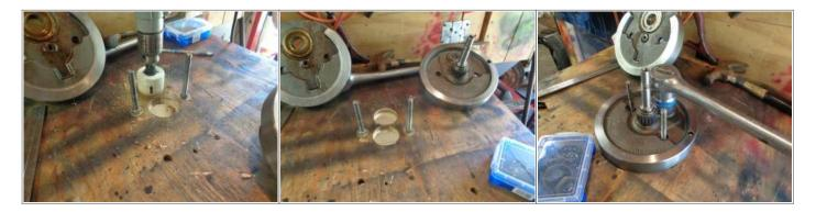
Then, knock the pin out with punch and hammer (make sure there is something soft under the crank pin for it to land on).
