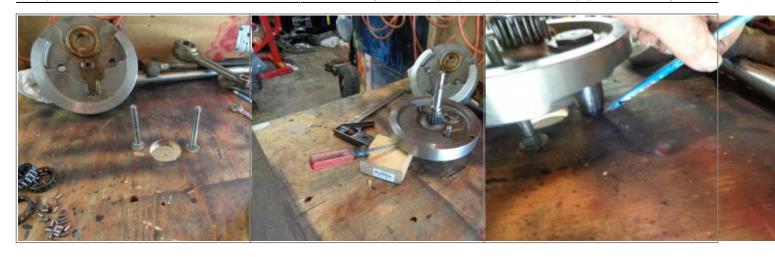
Then another 2" hole was made into the outline for the crank pin. Lower the wheel into position and the nut can now be removed with the 1-5/16" socket.
