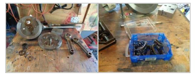
Next, the jig has to be drilled to accept the crank pin and allow the bottom flywheel to sit over the holding pins.
