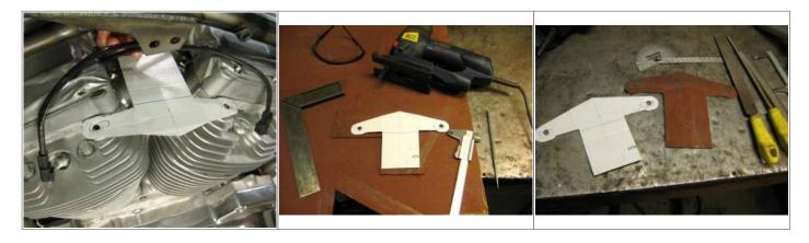
A breaker tool was fabricated in a hydraulic press to make 22.5° degree bends on each lug for the mount.
