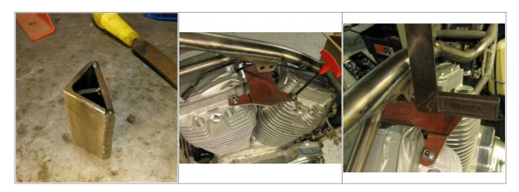
The mount was placed over a small vise (with the jaws opened and the edges rounded to help the bending process of the mount material).
