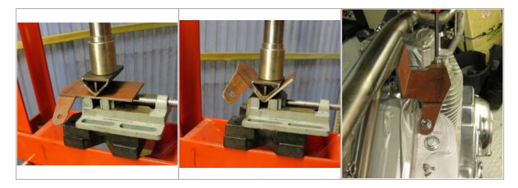
Then two gussets were fabricated using the above method of bending and then welded to the mount on both sides. 4)
