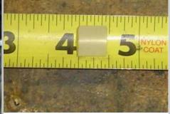
On 57-03 engines, you can carefully screw a bolt into the timing hole until it snugs up against the flywheel. You can also place a piece of polyethylene tubing in the
