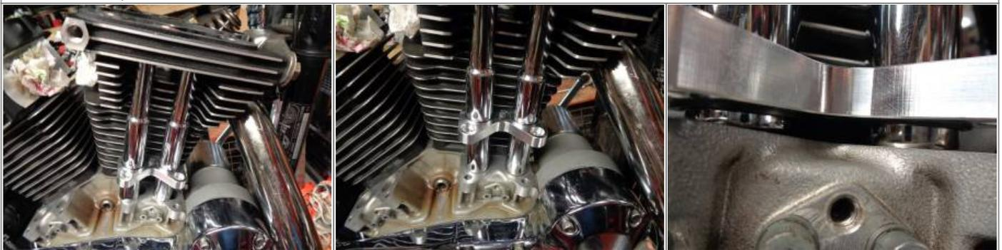
**Check the clearance between the tubes and cylinder fins before installing the bolts.**
