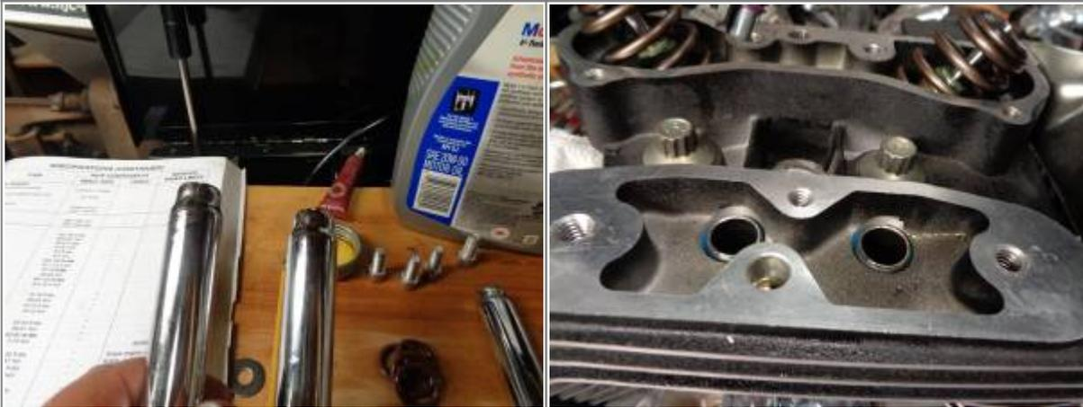
Swing them in and center the tubes over the lifter bore. Stop short of all the way down and make sure the seals are still in place all around the base.
