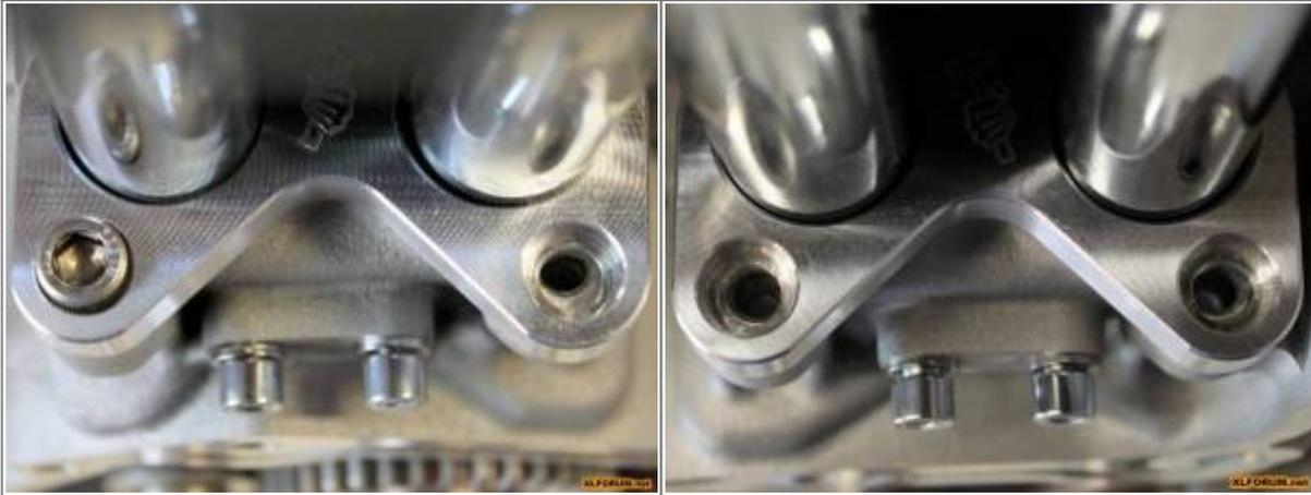
Also check that the cylinder base gasket isn't interfering with the pushrod tube base. <sup>15)</sup>
