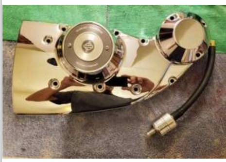
Hayden KVP38 breather valve, used with the Deimus Mod (cam chest breather conversion). 26)
