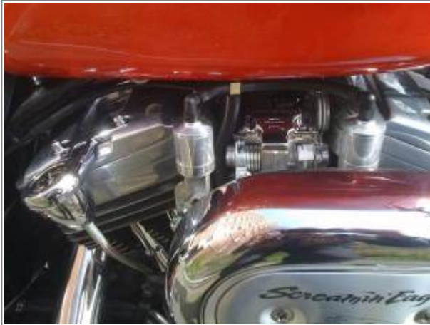
Hayden KVP38 breather valve, used with the Deimus Mod (cam chest breather conversion). 26)
