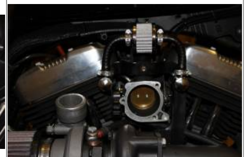
Filter mounted high will receive built up sludge. 10)
