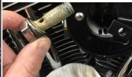
Rear bolt covered in sludge. 9)
