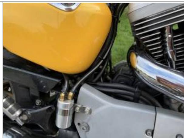
The tube from the catch can runs up under the fender and exits at the rear on the left side of the bike. When the bike is on the jiffy stand the hose is way over the side.
