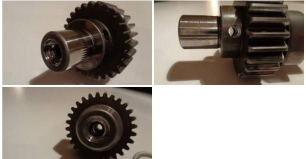
The hole in the outside end of the cam is for the breathing, it is the sole exit for the engine pressure. Air from that hole in the cam will go to an external reed valve. The original breather exit in the cam-case (4-speed) is to be plugged off.
