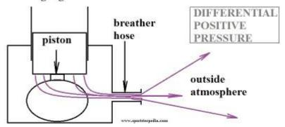
With the piston falling, air is pushed by the piston. The pushed air pressure is higher than the atmosphere outside the engine. We refer to this as a pressure condition inside the engine. With / without the breather valve inline, air is pushed out of the engine. Also expressed as a positive pressure. Also measured with a PSI gauge.
