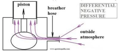
With the piston rising, air is pulled up under the piston. The pulled air pressure is higher than the atmosphere outside the engine. We refer to this as a vacuum condition inside the engine. If there were no breather valve inline, atmosphere would be pulled into the engine. Also expressed as a negative pressure. Also measured with a vacuum gauge.
