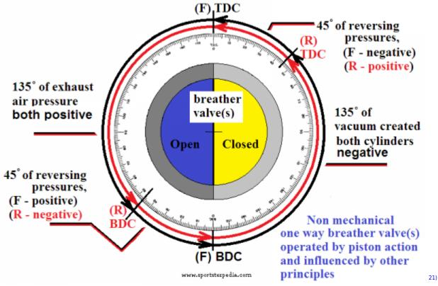
**1972-1976** Sportster Crankcase Pressure Cycle One crank rev shown, front cylinder, w trailings from rear cylinder
