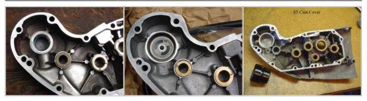
91-up engines breath from the heads instead of the cam cover but the principles are the same. The drain hole in the 98 chamber appears to be slightly bigger than that in the cam covers.
