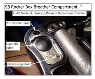
In 2004-up engines, the umbrella was encapsulated in a plastic housing (removing the need to create the separation chamber in the rocker box casting).
