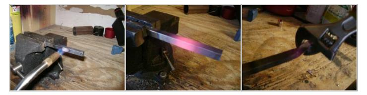
The first bend below twisted OK but the rod bent some.
