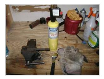
Start with some square stock. Mount it in a vise and pre-size an adjustable wrench to the bar so you can grab it without wasting time and letting the metal cool. <sup>2)</sup>
