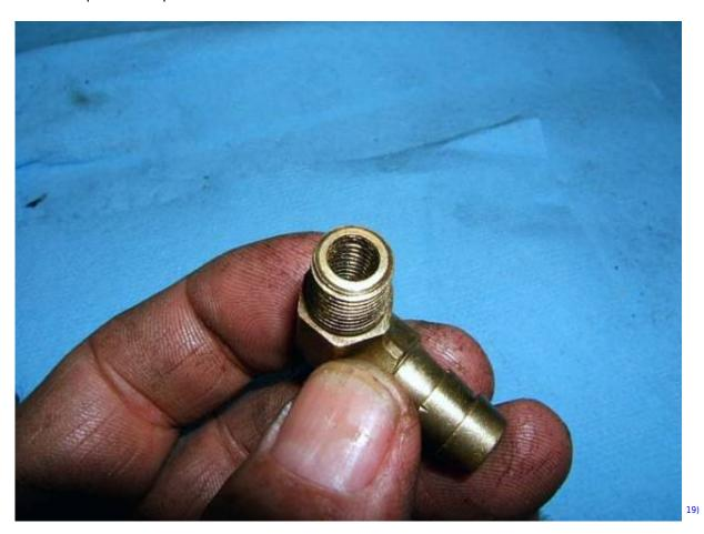
• Here, I've put Teflon tape on the threads and also screwed in the jet (never mind that it's a 170, it's all I had handy for taking these photos). Loctite red on the threads of the jet wouldn't be the worst idea in the world, and tighten it good.
