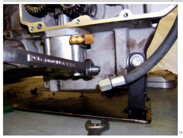
• After the hose is removed, remove the flare fitting from the pump body.
