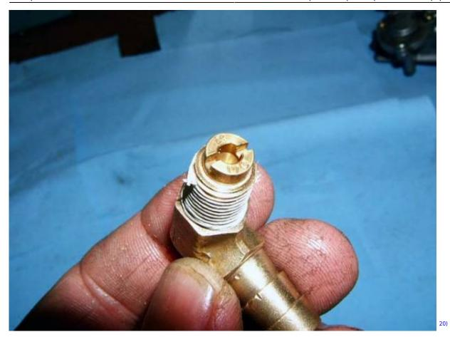
• Install this fitting with the jet onto the street tee as shown.
