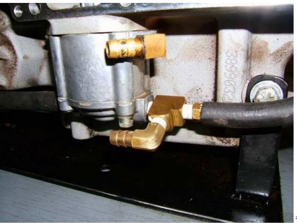
• Now prepare the 1/4" pipe thread fittings as shown. You probably could do all this with 1/8 pipe instead, and it'd be smaller and more compact. I chose 1/4 just because it's important to keep the restriction in the scavenge section minimal. But I'm probably worrying about nothing.
