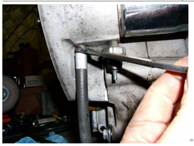
• Replace it with a 3/8" hose barb fitting. Teflon tape can be used on the threads, but in theory, a brass fitting into aluminum shouldn't need it.
