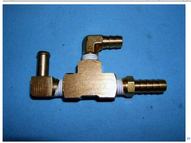
• Install the prepared 1/4 pipe tee and plumb as shown. Use hose clamps though, I was just mocking this up so I didn't bother. Tighten them all securely.
