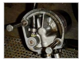
If you're using a check valve, the 86-90 oil filter adapter must be used. The check valve in 85 and prior models is in the oil pump. Therefore, the filter adapter is not set up for the check valve.
