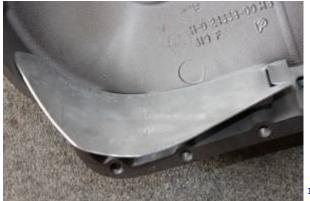
To re-direct the oil to the front of the sump, a raised expanded mesh was cut to make a pattern. Then the actual piece was cut out of mild steel (so it can be welded).
