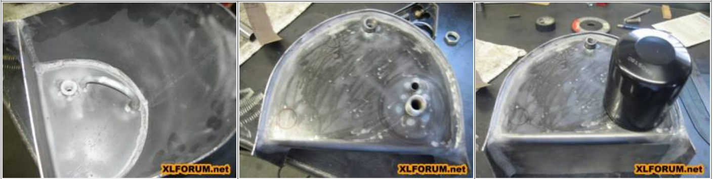
Filter mounted onto oil tank. The return oil goes through a loop inside of tank, back out through filter and returns through center of filter. 40)
