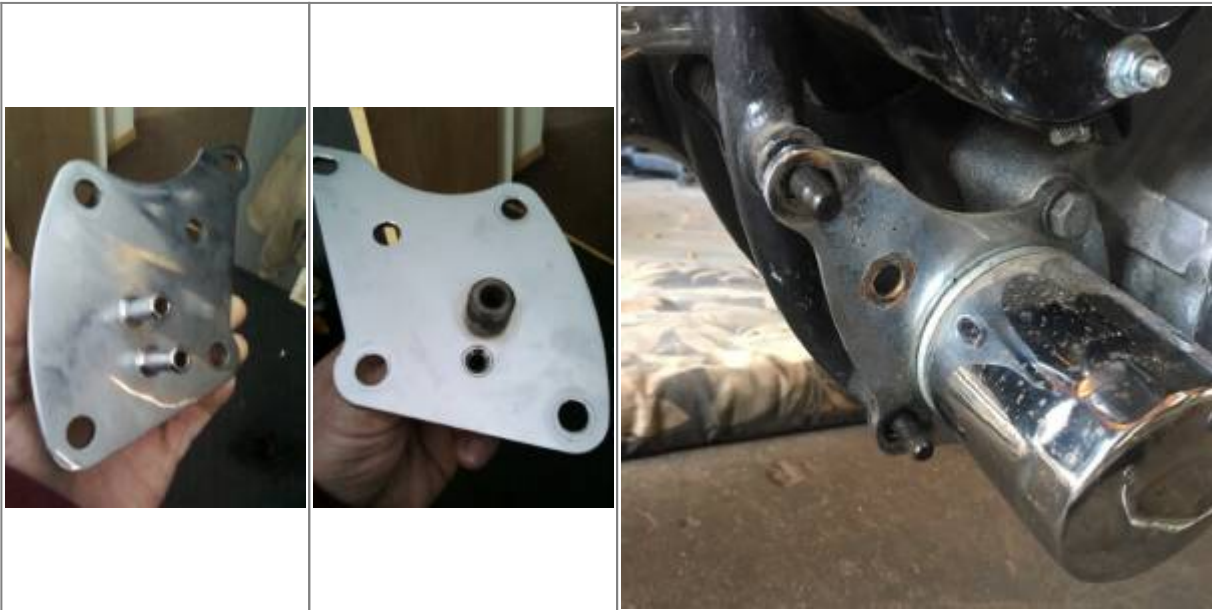
Motor mount oil filter on 69 XLCH 23)
