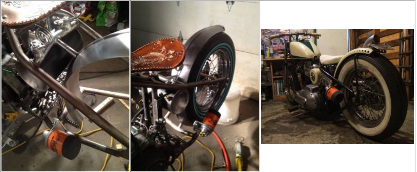
Custom oil filter mount on an 81 XLH 34)
