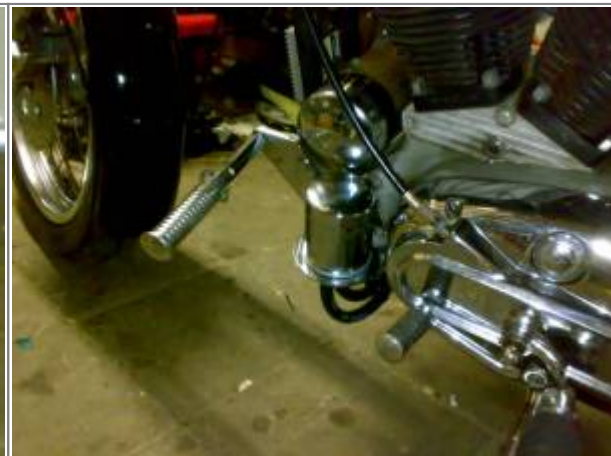
This one sets the filter upside down. 26)
