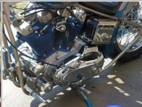
Filter installed on 77 XLCH motor mount. 24)
