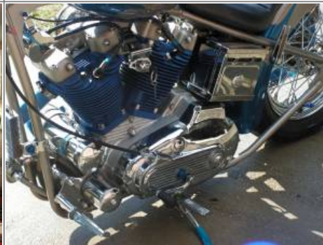
Filter installed on 77 XLCH motor mount. 24)
