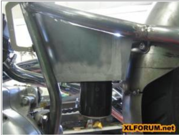
Filter mounted onto oil tank. The return oil goes through a loop inside of tank, back out through filter and returns through center of filter. 37)
