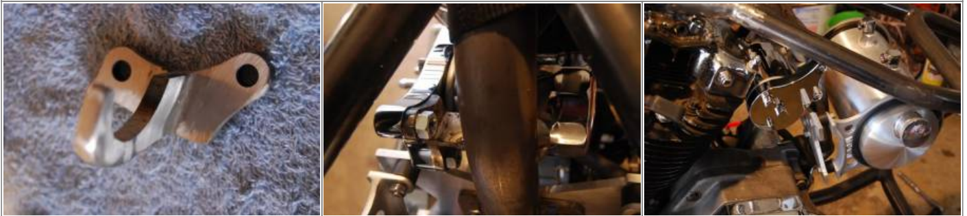
Custom built oil filter mount. 31)
