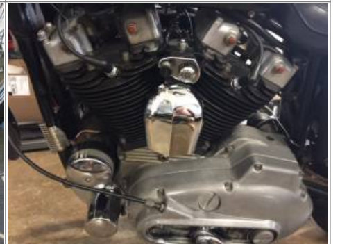
Filter installed on an 80 XLH motor mount. 25)
