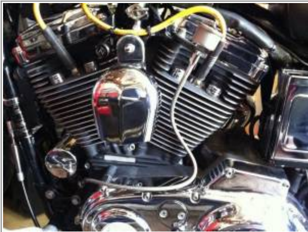
Remove the oil filter and oil pressure switch. 11)
