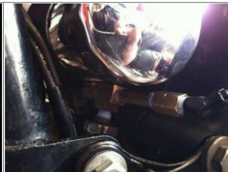
2nd 90° faces down to mount the oil pressure switch. Measure to position the fittings so the switch is clear of the frame and engine case. 14)
