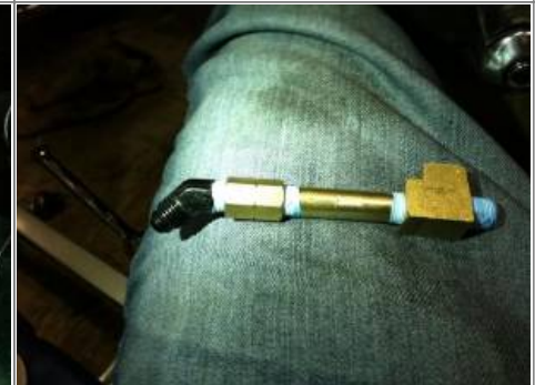
2nd 90° faces down to mount the oil pressure switch. Measure to position the fittings so the switch is clear of the frame and engine case. 14)
