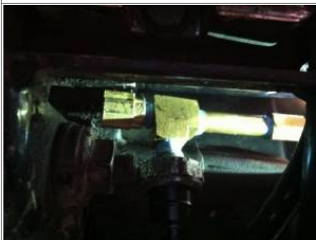
2nd 90° faces down to mount the oil pressure switch. Measure to position the fittings so the switch is clear of the frame and engine case. 14)
