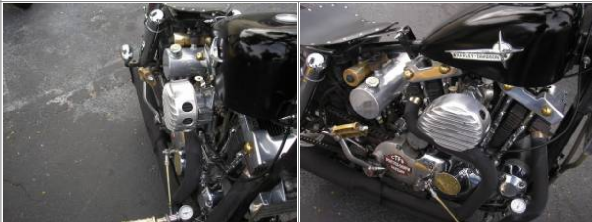
Oil pressure gauge on a 74 model mounted down low by the forward controls 24)
