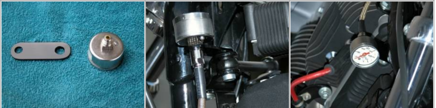
Gauge mounted on the enricher bracket with an L shaped bracket from an old carb support. 36)
