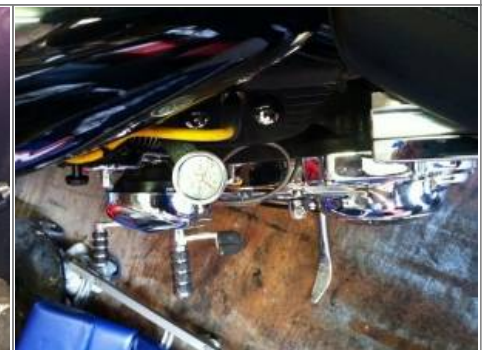
2nd 90° faces down to mount the oil pressure switch. Measure to position the fittings so the switch is clear of the frame and engine case. 14)
