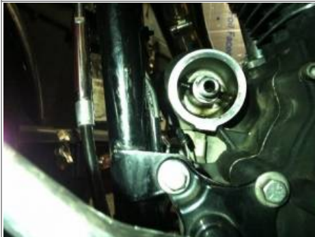
2nd 90° faces down to mount the oil pressure switch. Measure to position the fittings so the switch is clear of the frame and engine case. 14)
