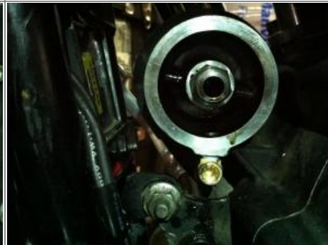
2nd 90° faces down to mount the oil pressure switch. Measure to position the fittings so the switch is clear of the frame and engine case. 14)
