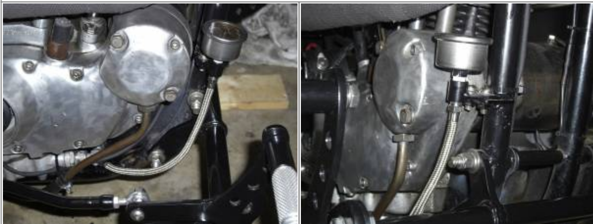
Oil pressure gauge on a 74 model mounted down low by the forward controls 24)
