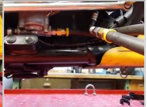
Hook the other end to the oil pump. 20)
