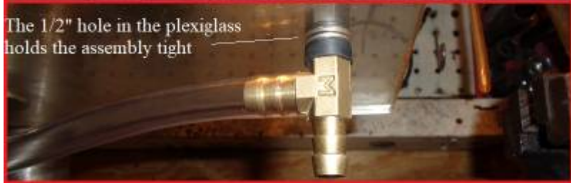
1 gallon water jugs tapped for oil lines. 1/8" x 27 holes tapped into 3/8" x 1" plexiglass blocks glued w/ clear Gorilla glue
