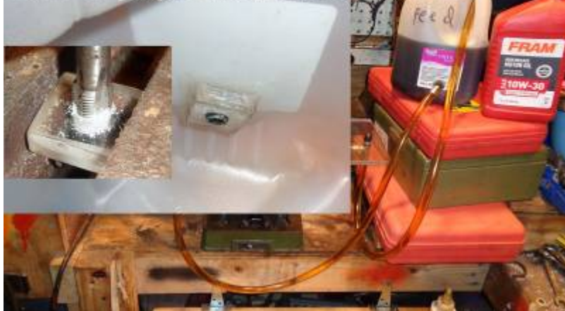
1 gallon water jugs tapped for oil lines. 1/8" x 27 holes tapped into 3/8" x 1" plexiglass blocks glued w/ clear Gorilla glue
