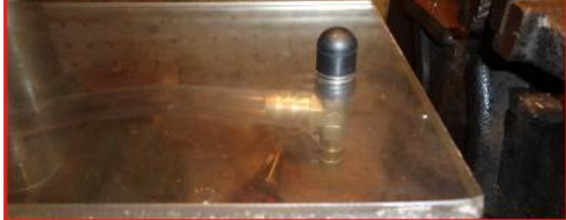
The 1/2" hole in the plexiglass holds the assembly tight
