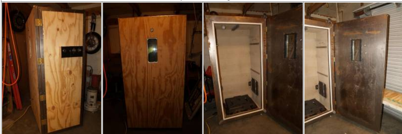
Homemade powder coating cabinet. 5)
