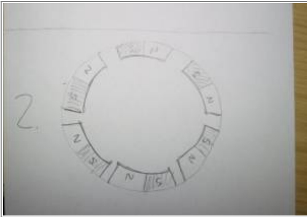
Correct magnet pole positioning 19)
