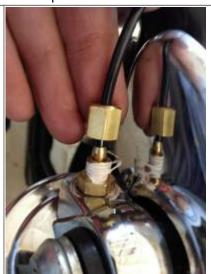
The Teflon tape isn't necessary as in the pic above. That's not what keeps it air tight. It's the ferrule that keeps it tight.
