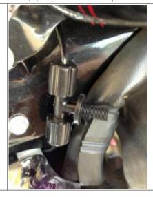
1-1/2" washer were used on the top and 2-1/2" washers on the bottom to clear the belt guard. Stock bolt was re-used.
