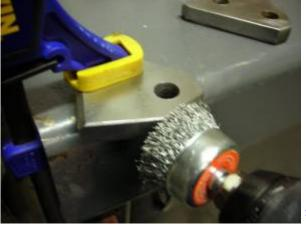
The final shaping was done, edges smoothed with a wire brush, test fitted and painted.
