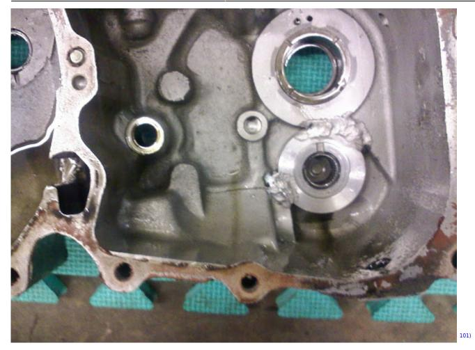
• This procedure results in no perceptible warpage at the case parting seams. this cant be said when the case corner is blown apart and a new cast corner piece is welded in. Obviously the outcome is dependent on quality of workmanship. When doing this work the time is right for making sure your door fits correct too. <sup>102</sup>
