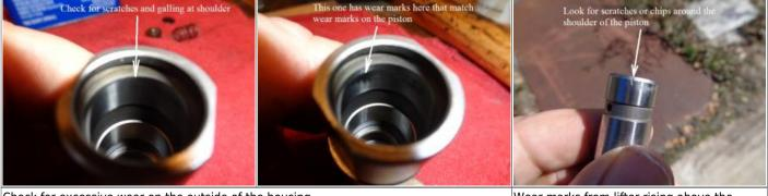
Check for excessive wear on the outside of the housing. Excess scratches should signal you to check the lifter bore clearance in the case.<sup>12</sup> Wear marks from lifter rising above the anti-rotation pin. <sup>13)</sup>
