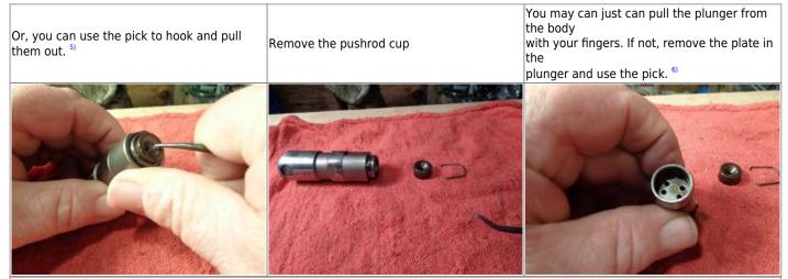
Once the plunger is out, turn the body upside down and let it drain. Pull the plate out if you haven't already.  $^{\prime\prime}$
