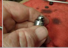
This plate, spring and cup make up the check valve for this lifter.<sup>9</sup>
