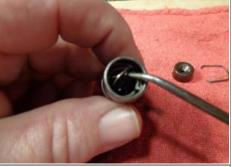
This is the lifter's check valve (some have a plate and spring, others have a ball and spring). The cup pries off with a screwdriver. Careful not to lose the cup or the tiny spring under it.<sup>8</sup>
