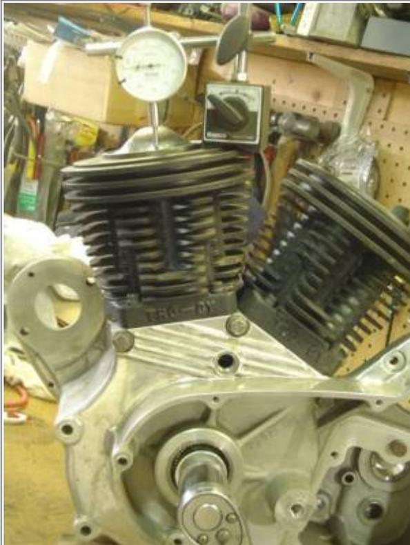
For Ironhead and Shovelhead cylinders, pull the head and install the indicator. <sup>6)</sup>
