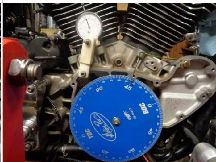
3. Continued rotation up / back down to .053" cam lobe height. Degree wheel shows: 46° after bottom dead center (ABDC) 14)
