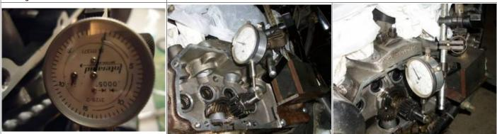
This gauge post is threaded into a cover mount hole.<sup>5)</sup>
