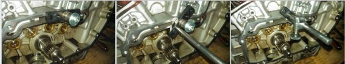
Install a dial gauge on the holder with the pointer on the pinion shaft. Find the lowest spot while turning the engine over and 'zero' the indicator. <sup>3)</sup>
