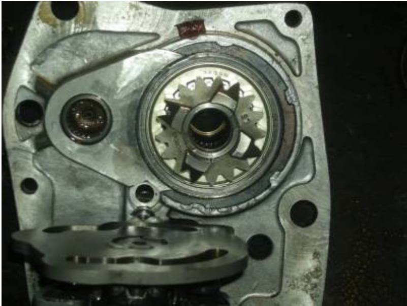
Clutch gear with new bearing loaded into trap.
