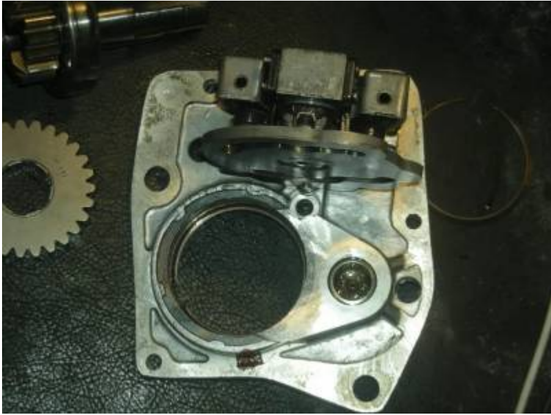
Clutch gear with new bearing loaded into trap.
