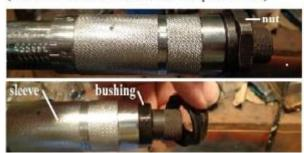
Install the nut, set the torque value again on the wrench and test the click point. You may have to do this and few times before you get the click point exactly on the mark
