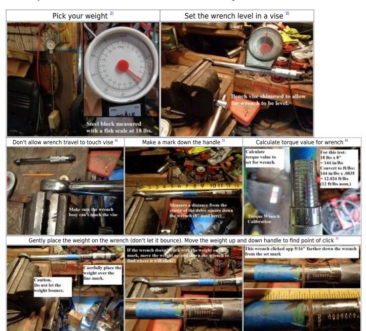
As a double check, more weight was added to test the wrench at a higher torque value of 22 ft/lbs. The results were about the same. App 3/8" down the wrench is where it clicked using 34 lbs. and the same 8" length. 8)
