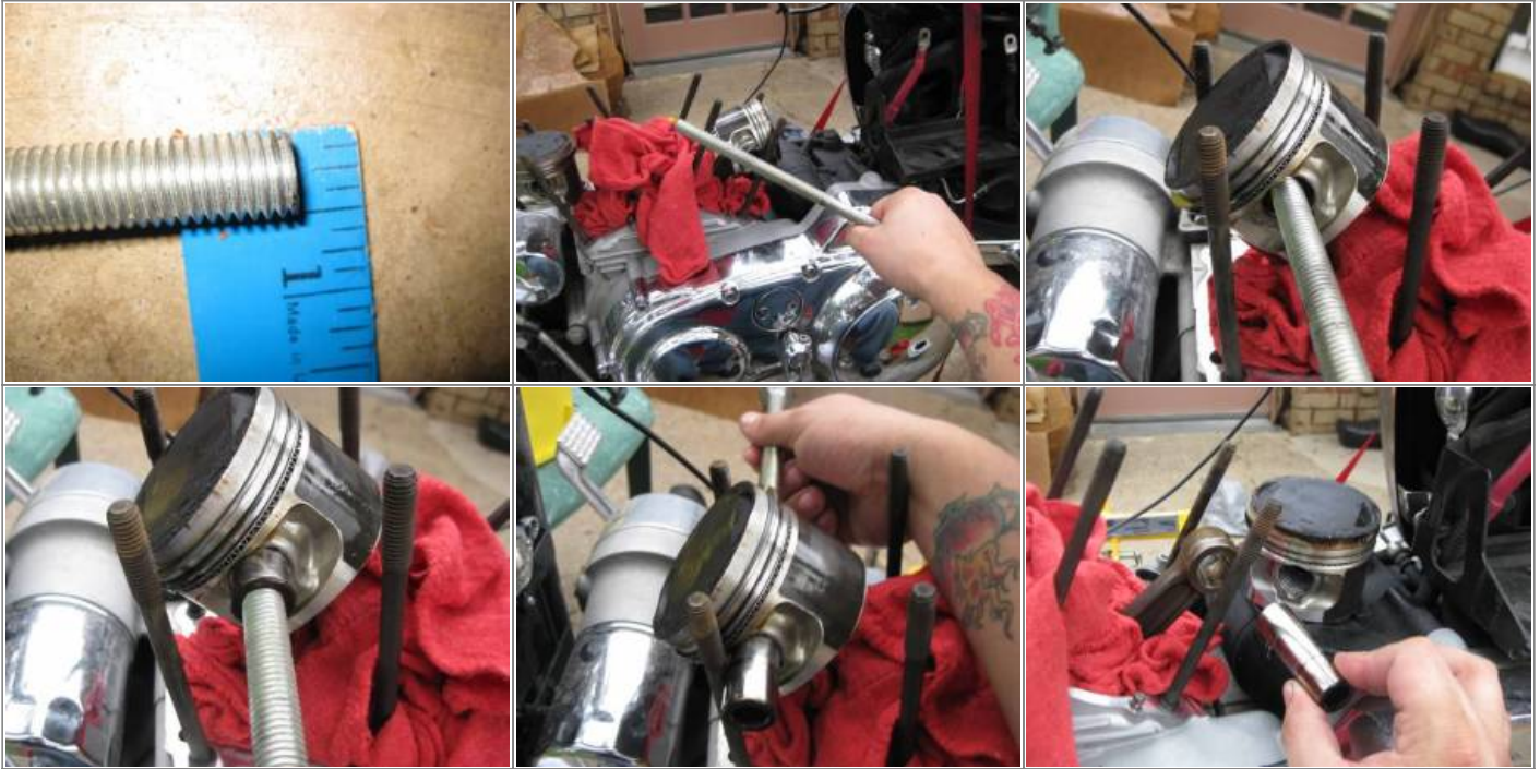
A 1/2x13 carriage bolt set into the pin hole and either pushed or light threading motion with pressure applied to remove the wrist pin. 8)
