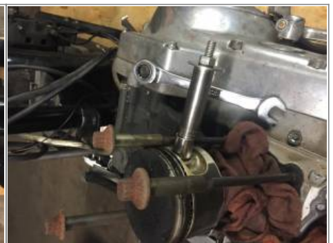
Home made wrist pin removal / installation tool. 5/16" all thread, 2 fender washers, two nuts, two PVC spacers and two 1/2" sockets. 4)
