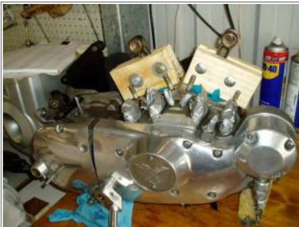
A couple bits of timber and four bolts. Holds them nice an steady for reaming. 9)
