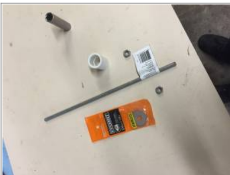
Home made wrist pin removal / installation tool. 5/16" all thread, 2 fender washers, two nuts, two PVC spacers and two 1/2" sockets. 4)
