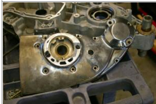
Modified cam covers for reaming 13) 14)
