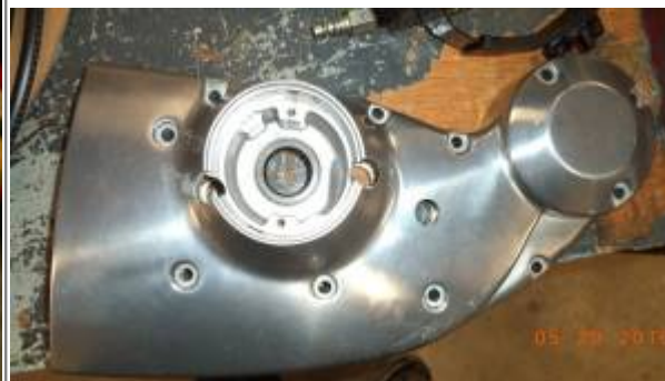
Modified cam covers for reaming 13) 14)
