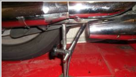
Camera mounted to a dial indicator magnetic base 1)
