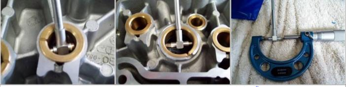
Telescoping bore gauge and caliper for measuring cam bushinhgs. 9)
