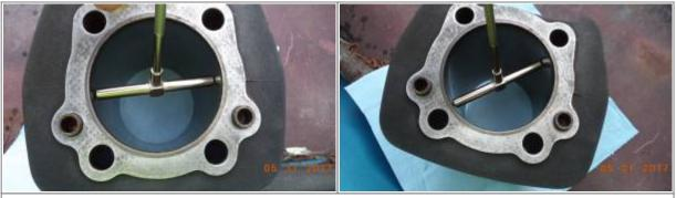
Measure around the circumference for accurate readings.
