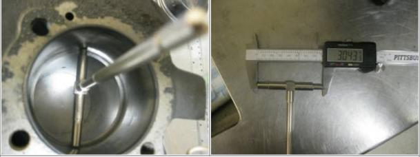
Telescoping bore gauge and caliper for measuring cylinder I/D. 8)
