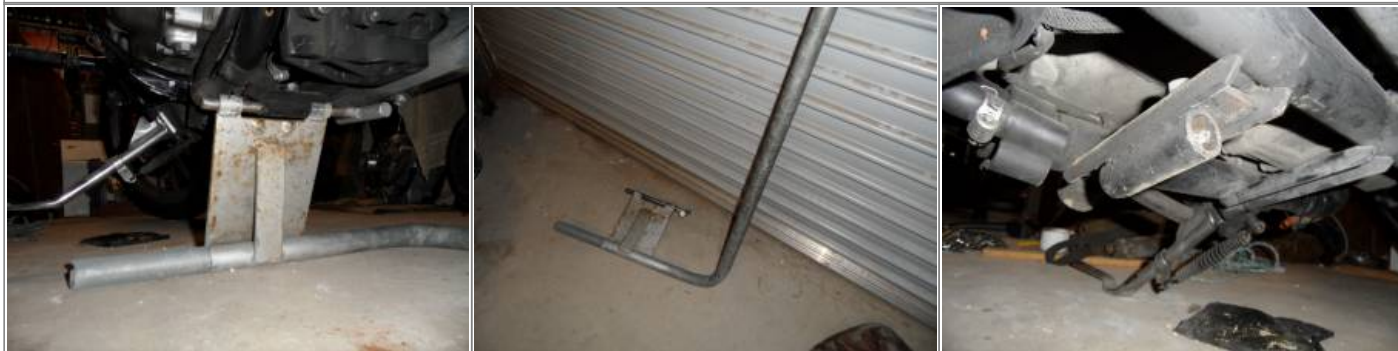
Homemade locking hand lift made one out of scrap and it doesn't need tie-downs. This makes the bike stable enough to sit on, work on and even have both wheels off at the same time. 11)
