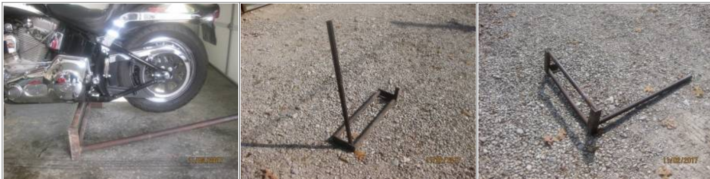
Homemade hand lift made of old steel pipe 10)
