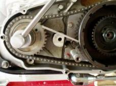
Two more little pieces to jam between the inner and outer clutch drums, with the main sprag still in place. You have to be careful to keep them all in position when tightening. <sup>6)</sup>
