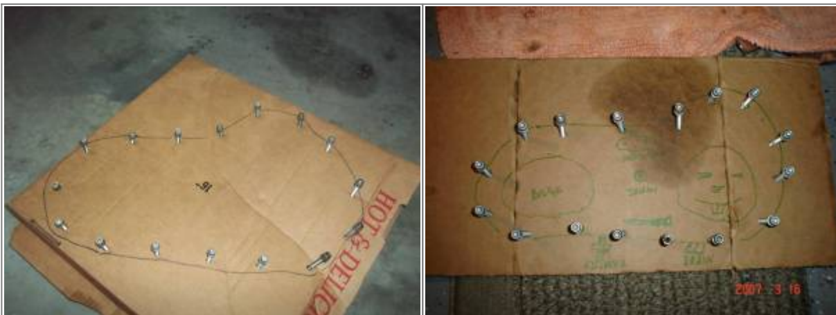
Protecting / retaining primary cover screws 7) 8)
