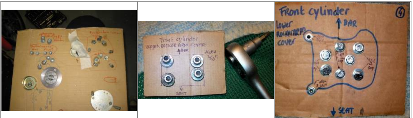
Protecting rocker box screws and parts 11) 12) 13)
