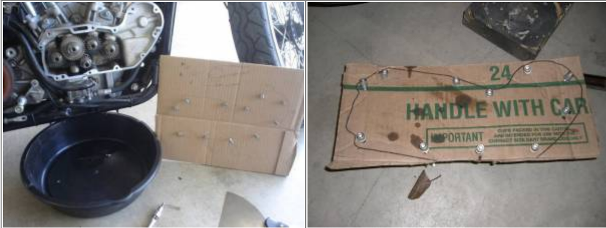
Protecting / retaining gearcase cover screws 9) 10)
