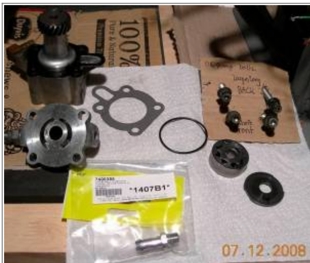
Protecting oil pump mounting bolts 16)
