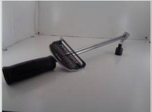
3/4" Drive - Beam Torque Wrench 9) Range: 0-300 ft/lbs
