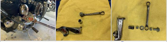
Dial type torque wrench with box end wrench extension. 19)
