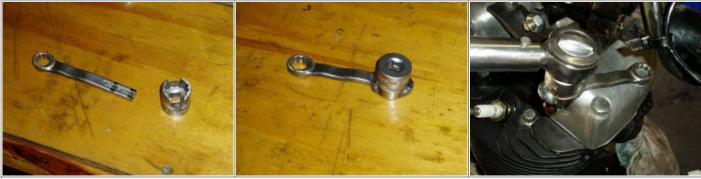
Homemade Wrench Extension for in-frame applications 15)
