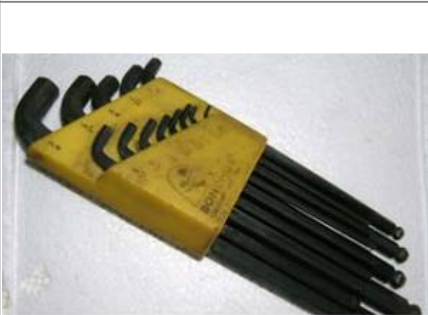
Bondhus makes some stubby hex key wrenches that are perfect for things like those lower intake manifold bolts.
