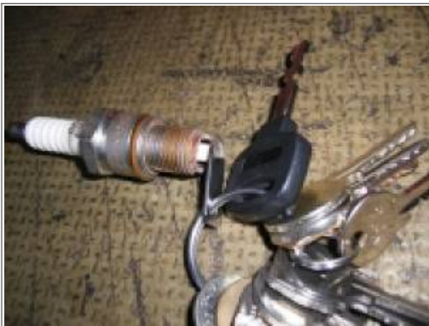
Homemade Spark Plug Gapping Tool 2)
