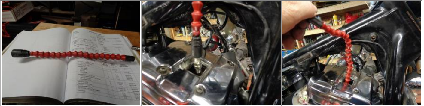
STEELMAN PRO 08310R flexible 12-Inch spark plug starter tool 5)
