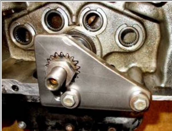
3/8" stainless steel plate with 20° spokes (for 18 teeth), sawed initial groove to depth and widened it with files
