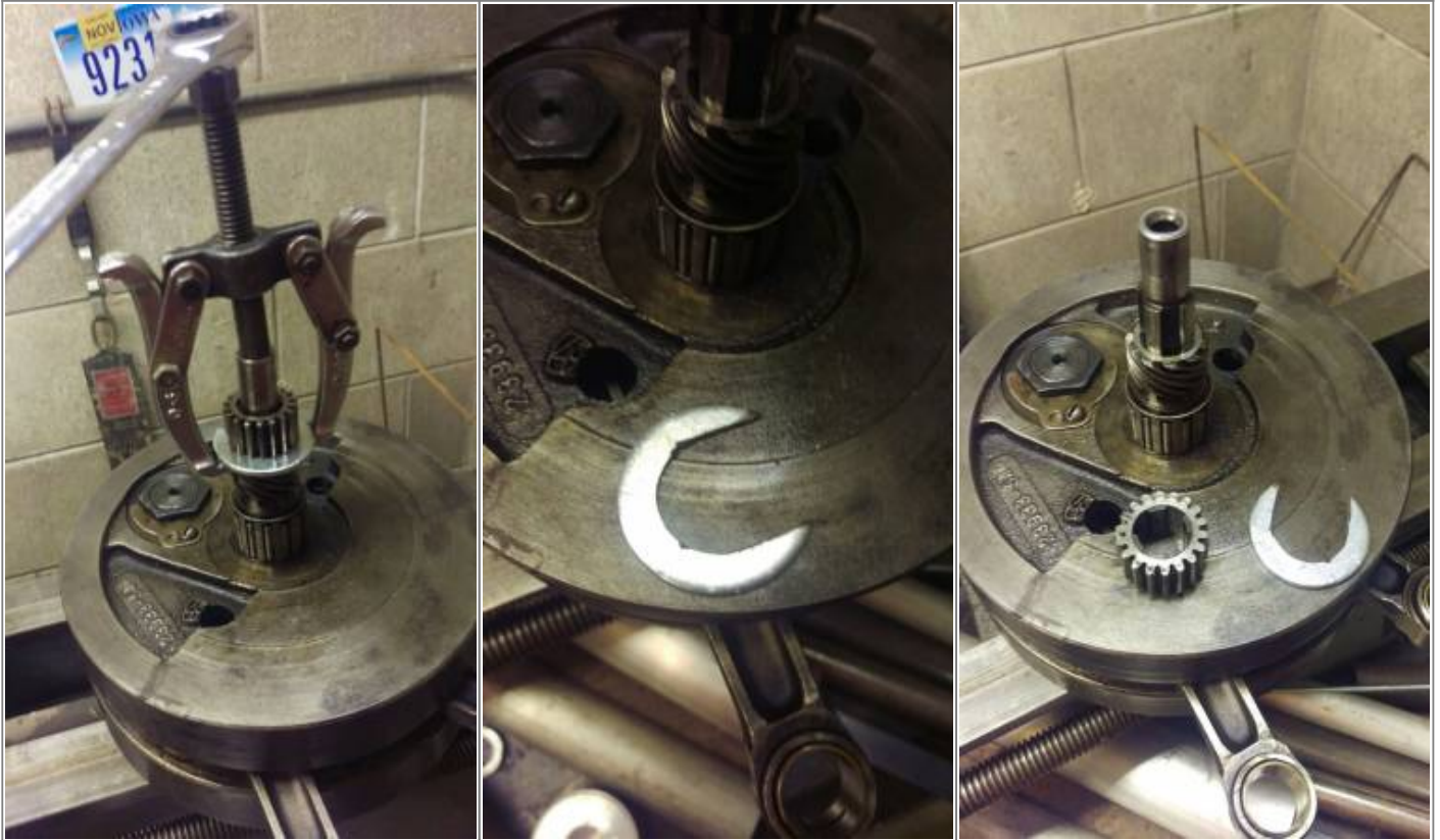
Large fender washer cut into a "C" shape and a gear puller
