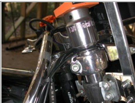
Squeeze the trigger to pull the cap down. 4)
