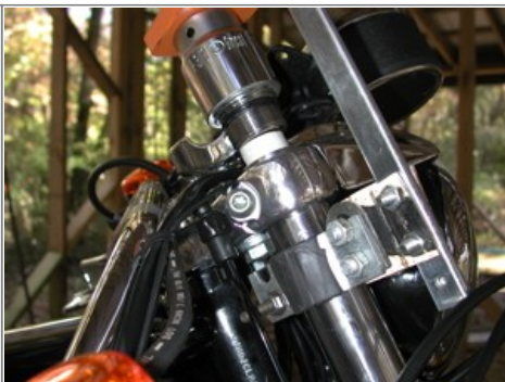
Squeeze the trigger to pull the cap down. 4)
