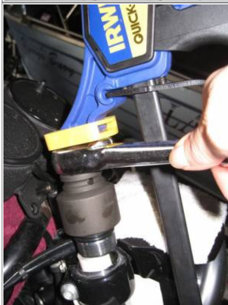
It may take a few goes to get it to depress squarely into the tube. Then just turn the socket until the threads on the cap start properly. 6)
