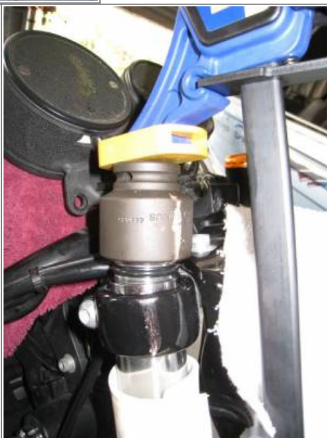
It may take a few goes to get it to depress squarely into the tube. Then just turn the socket until the threads on the cap start properly. 6)
