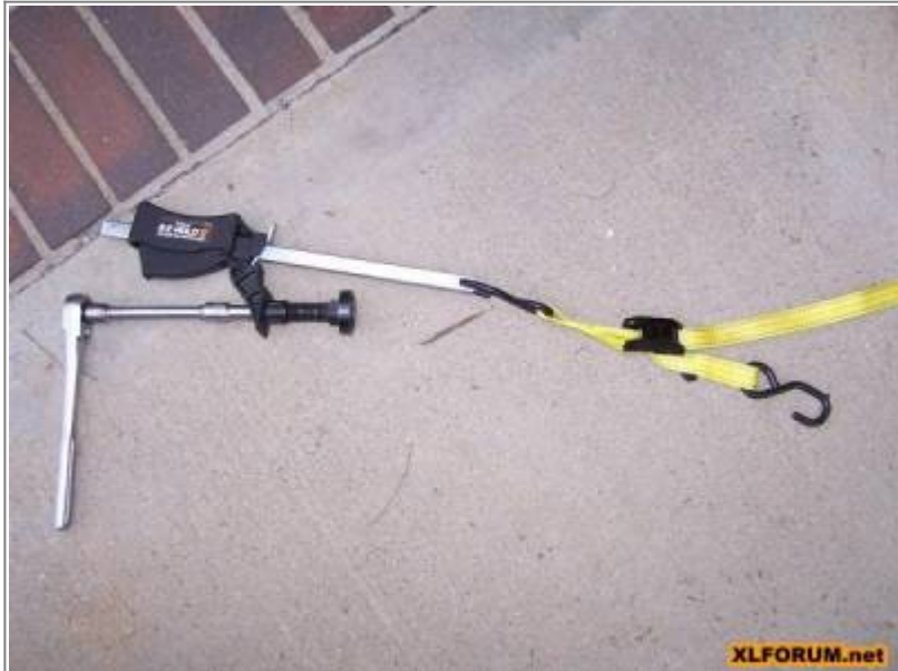
Homemade fork spring compressor 8)
