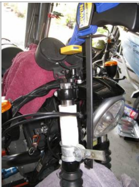
It may take a few goes to get it to depress squarely into the tube. Then just turn the socket until the threads on the cap start properly. 6)
