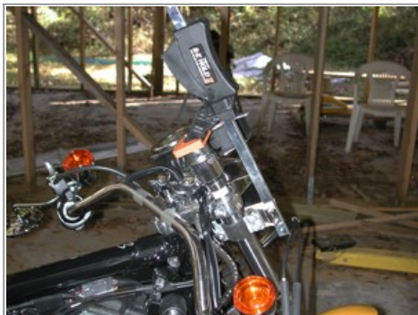
Attach the conduit clamp to the fork. 3)
