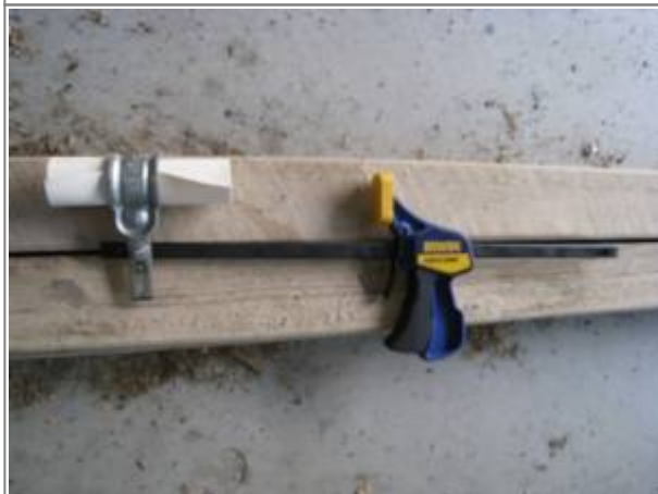
Homemade fork spring compressor 5)
