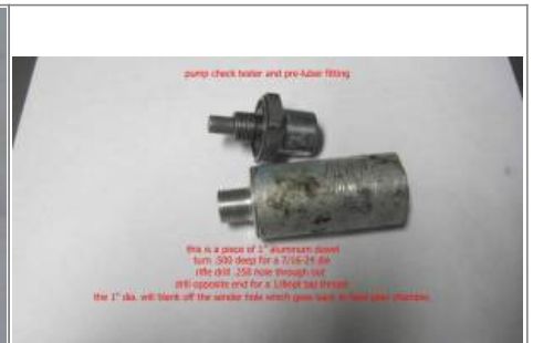
Oil pump check valve tester / pump prelube tool. 6)
