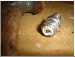
You'll need to tap threads into the gutted out portion of the plug. In order to get good threads in the plug body you need a bottoming tap (no taper).
