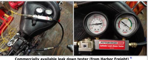
Commercially available leak down tester (from Harbor Freight) 3)
