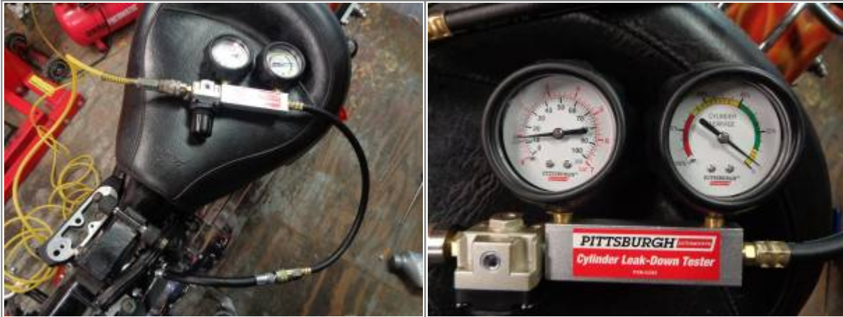
Commercially available leak down tester (from Harbor Freight) 3)
