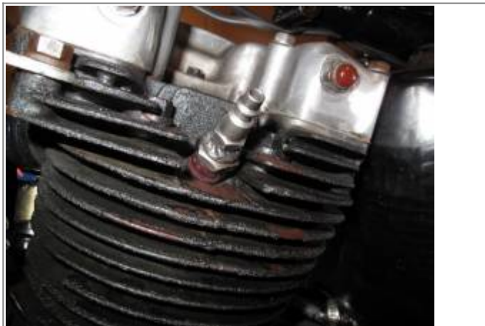
Homemade air nipple welded into the plug. 8)
