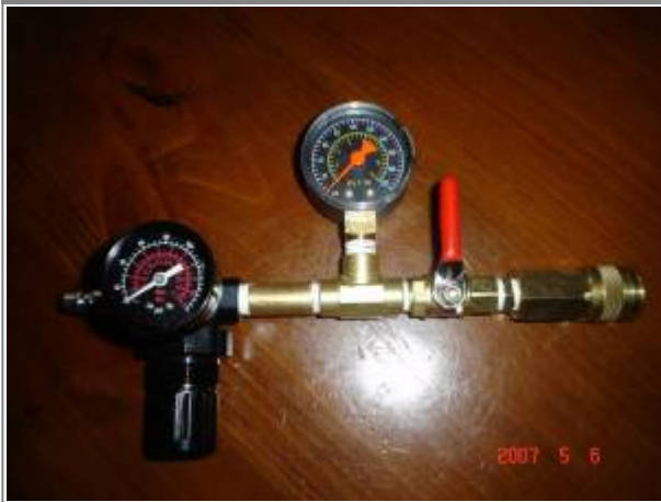
Homemade Leak-Down Tester 4)
