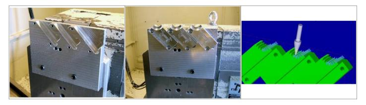
The table turns to one angle and cuts one tooth on each block. Then the table turns to another angle and cuts one tooth on each block, etc.
