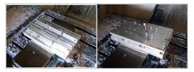
**Step 3**Each tool is cut out of the material block, engraved and the pieces are faced off (clean straight ends).
