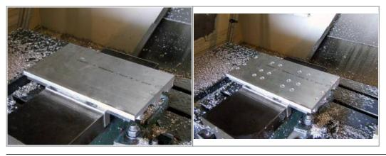
This jig was made to allow each tool to be cut from the material block.
