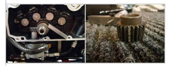
I torqued the pinion gear to 70 ft. lbs. using a tool I made just for this purpose (below). I had another friend of mine scribe "HAMMER PERFORMANCE" on it and then sent it to Hammer Dan as a token of my appreciation for all of his help. <sup>3)</sup>
