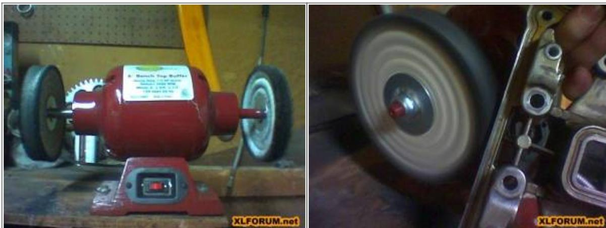
Polishing a rocker box top with a benchtop buffer <sup>2)</sup> <sup>3)</sup>
