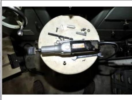
High speed grinder and hard felt wheel <sup>10)</sup>
