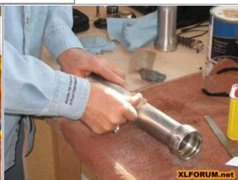
Filing the fender mounts off the fork sliders 3)
