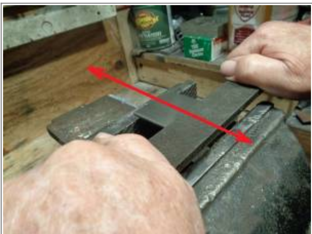
Draw filing stainless steel with a bastard file 7)
