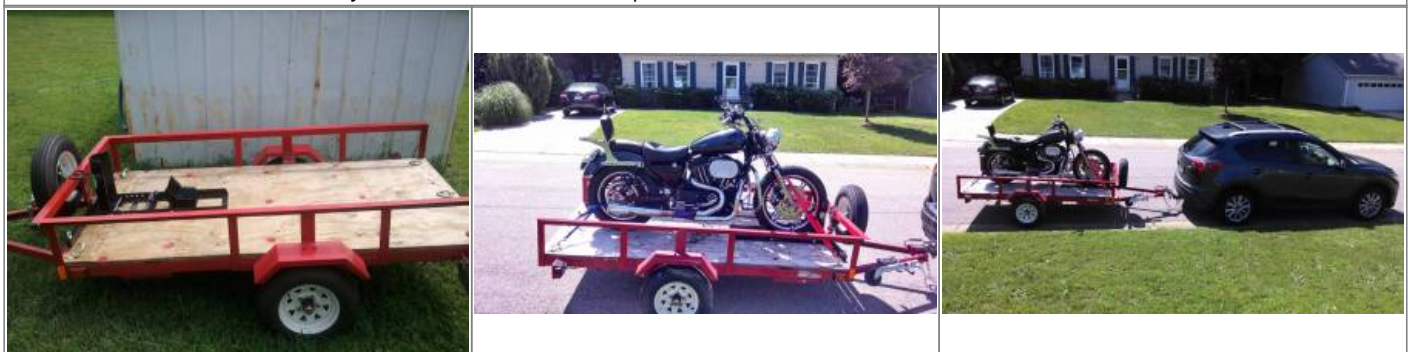
4x8 heavy duty Harbor Freight trailer w/ added rails, all bolted joints welded and a plywood bottom. 16) 17)
