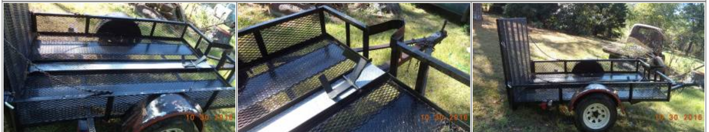
1/2 Ton Utility Trailer modded with walk panels, tire channel, wheel chock & front tire shroud 15)
