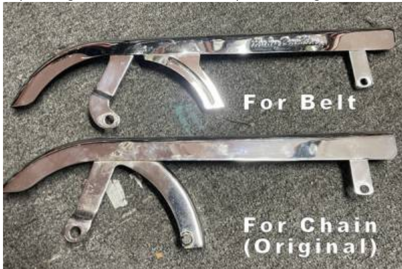
Top: Belt guard ——— Bottom: 4 speed chain guard
